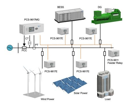
Note: When the microgrid capacity is small, the local controller could not be configured and the microgrid controller communicates directly with DG, energy storage and diesel engine.
