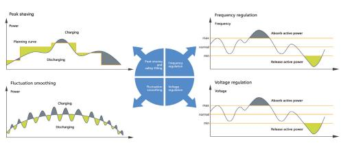
PCS is the interface between grid and storage system, which can store the electrical energy from grid into the energy storage device as well as release the energy into the grid from the storage.
